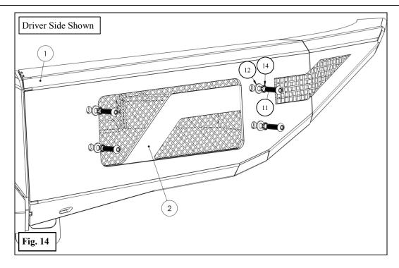
12. Align bumper as desired and torque all hardware as specified: M6 to 7 ft-lbs, M8 to 18 ft-lbs, M10 to 38 ft-lbs, M12 to 60 ft-lbs.
