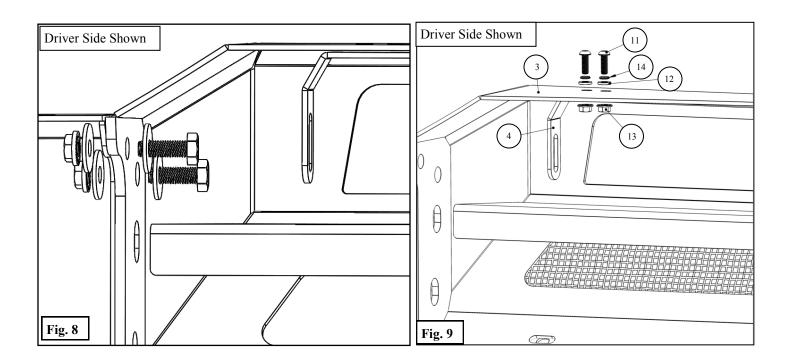
8. Loosely install the bumper assembly to the Mounting Brackets (5,6) using the supplied M12 Hardware. See **Figures 10,16.**
