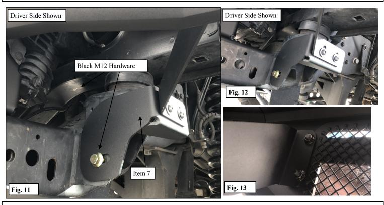
11. Attach the Mesh Side Covers (2) to the Bumper and Side Straps (9,10) using the supplied M6 Hardware. See **Figures 13 & 14.**
