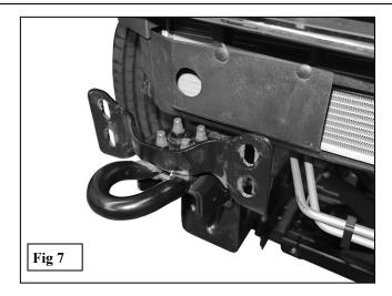
5. Remove the passenger/right side tow hook from the end of the frame, (Figure 7). Next, remove the (4) factory hex nuts, lower frame extension and double bolt plates from the end of the frame, (Figures 2 & 7). Repeat for Driver Side.
