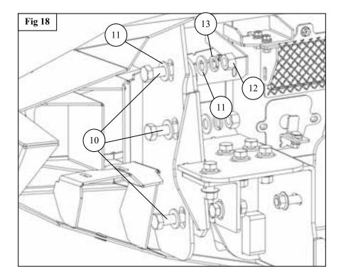
20. Adjust the bumper as needed and torque hardware as specified: M6 to 5-7 ft-lbs, M12 to 50-55 ft-lbs, M14 to 90-95 ft-lbs
