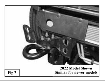
6. Remove the passenger/right side tow hook from the end of the frame, (Figure 7). Next, remove the (4) factory hex nuts, lower frame extension and double bolt plates from the end of the frame, (Figures 6 & 7). Repeat for Driver Side.
