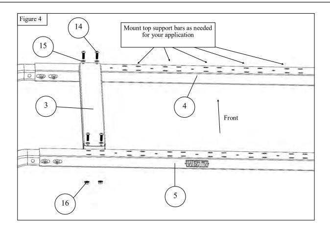
Align rack as necessary and torque hardware as specified: M8 to 15-18 ft- lbs, M10 to 35-40 ft-lbs. Note: The Overland Cargo Rack is designed to hold specific aftermarket accessories for the off road enthusiast, including roof top tents. Please see manufacture's installation instructions for mounting other accessories.
