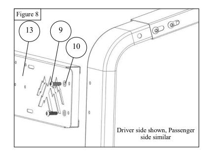
8. Using M8 hardware, mount the 2 top support brackets to the rack assembly. Note: The top support bars can be aligned as needed for your application. See Figure 9
