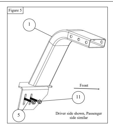
6. With assistance, loosely install the rear assembly near the cab using M8 hardware. See Figures 6-7
