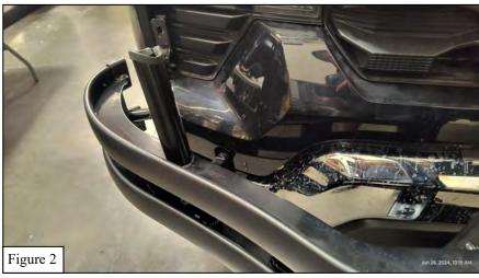
4. Mount the wing wraps using M10 Hex socket button head hardware (Items 5-7), M12 Hex socket button head Hardware (Items 8-10), and M6 Hex socket button head hardware (Items 11-14). See **Figure 5-8.**
