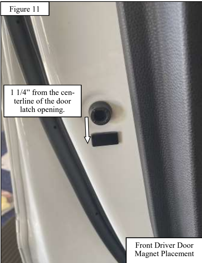
Front Driver Door Jamb Magnetic Induction Module Placement
