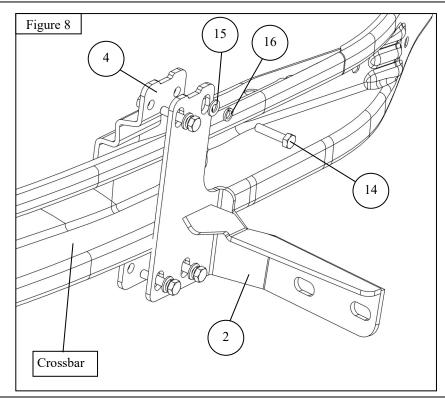
8. Measure the tips of the front mounting brackets. Make sure they are spaced around 25.75" inside between brackets and centered to the vehicle . See Figure 9
