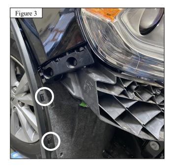
3. Unplug running lights before completely removing the fascia on each side. See Figure 4
